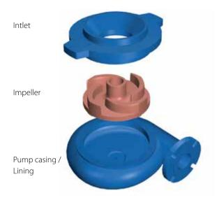
Standard pumps are supplied with parts in wear resistant Natural Rubber or High Chrome iron alloy, with a nominal hardness of 600 BHN.
