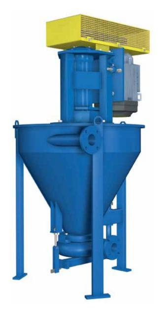
The pump, pump box, and motor, are integrated in one self-contained unit. Simple to install and connect. No alignment or special foundations needed.
